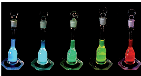
Figure 1. Fluorescence of methanol solutions of PPE-Ar-SO 3 − ( 14 ) under illumination with near-UV light. From left to right: Ph, Py, Th, EDOT and BTB. (From Ref. [48].)
